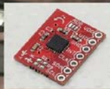
Arduino Triple-Axis Digital Output Gyro Sensor
